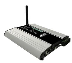
HSM240E-SD, the Swiss knife of modems, provides the added benefit of local control and monitoring and can work with Ethernet, serial, and digital I/O simultaneously. Besides this flexibility, the modem also supports standard Wi-Fi communication with selectable RF speeds up to 54Mbps in standard mode and 108Mbps in turbo mode for point-to-point and point-to-multipoint communication.
